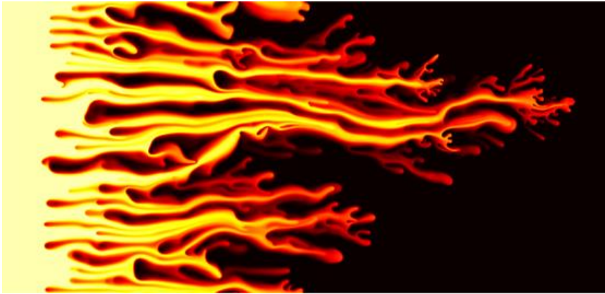
Figure 15. Snapshot of the concentration field during the unstable displacement of a more viscous fluid (dark) by a fully-miscible, less viscous fluid (light) ( http://news.mit.edu/2011/fluid-mixing-0519 ).
