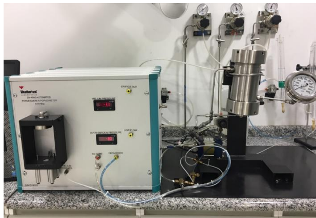
Figure 42. LRAP's porosimeter and permeameter. Source: LRAP .
