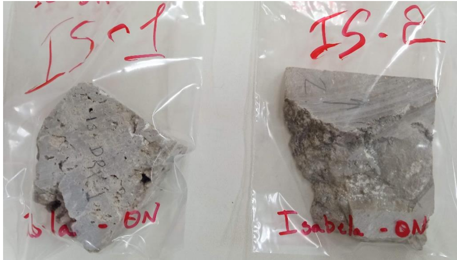
Figure 39. Samples analyzed by XRD; IS-1 (left) represents the vuggy facies and IS-2 (right) represents the laminated/massive facies.
