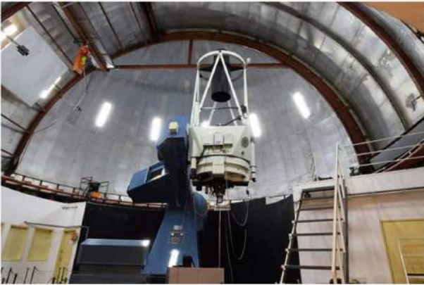
Figure 1. The 1.60-m P&E telescope and its dome at the OPD/LNA in Brazil. Picture credit: Saulo Gargaglioni, coordinator of the OPD/LNA.
