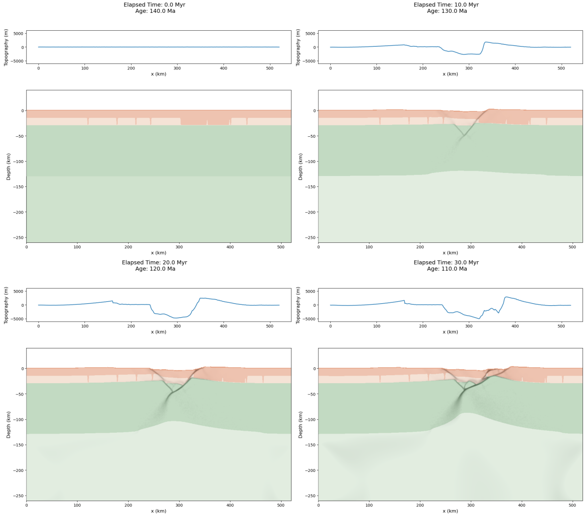
Figure 5.7: Accumulated strain, and topographic plots of the Model FM2. Dark and light orange represent the upper and lower crust, respectively. The vertical, thin, dark orange structures represent the shear zones, and the dark orange rectangular structure represents the Proterozoic Terranes. Dark and light green represent the lithospheric and sublithospheric mantle, respectively. Shades of gray correspond to the accumulated strain.
